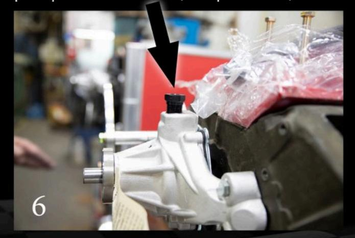
**3** | Hold the regulator in place and test fit your hoses. (See Photo #7) \*\*\*NOTE - Due to the high demand on your performance cooling system it is highly recommended that silicon hoses with the proper clamps be used. It's also recommended that a hump hose be installed to compensate for misalignment, vibration and or chassis flex. (See photo #8) Should you need a custom hose Art's Radiator has silicon 45 & 90 degree hoses as well as aluminum mandrel bent tubes. We can meet your demands
